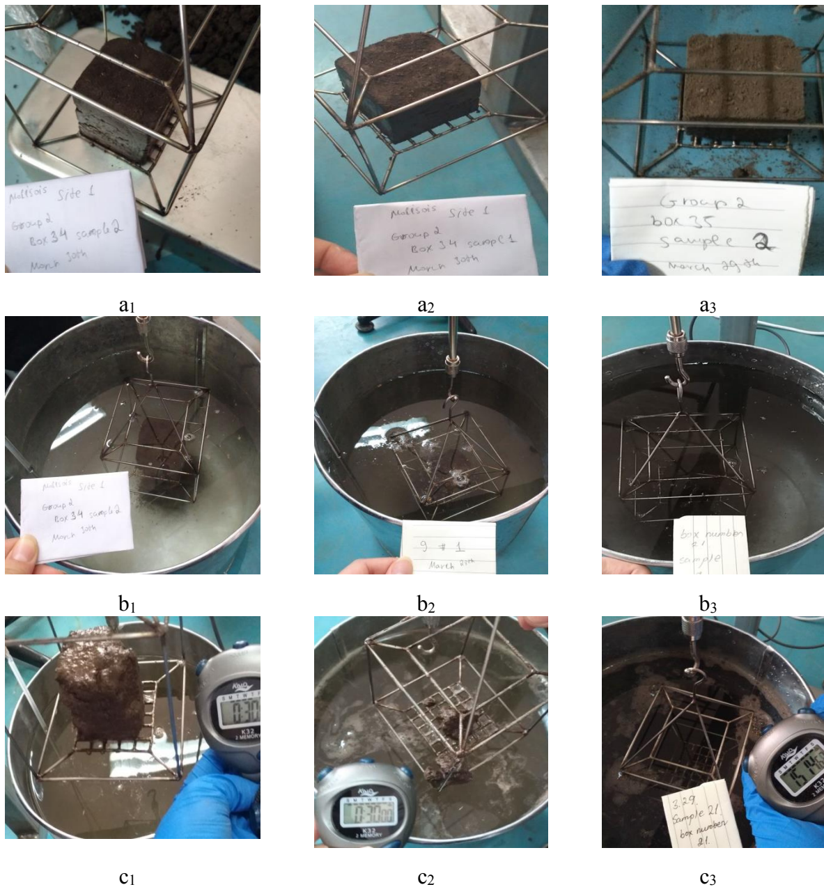
Figure 3-4 The main soil disintegration process with different initial soil water contents (a. 33.0% of SWC, b. 24.8% of SWC, c. 16.5% of SWC)
