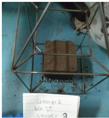
Figure 4-1 The main procedure of testing soil disintegration.
